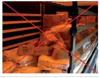
Preloaded cargo inadequately secured
